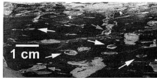
Figure 4: Polished slab of black shale bed from the Dowelltown Member, showing abundant "mantle and swirl" type bioturbation features (arrows). White arrows point to features that show predominantly the "mantle" character, and gray arrows point to features that display well developed "swirl" characteristics.
