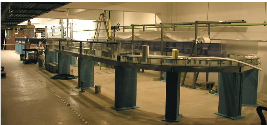
Figure 1: The current flume lab at Indiana University contains two racetrack flumes for the simulation of mud deposition and erosion.
